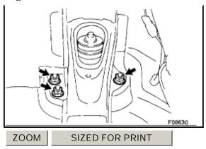
7. REMOVE REAR SHOCK ABSORBER Remove the 3 nuts and rear shock absorber. Torque: 80 Nm (816 kgf.cm, 59 ft. lbs.)
