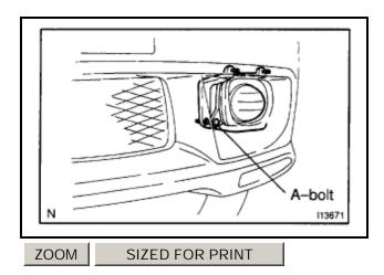
ADJUST FOG LIGHT AIM A-bolt: Vertical Direction
