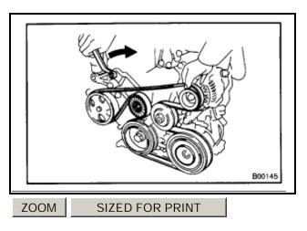
1. REMOVE DRIVE BELT Turn the drive belt tensioner slowly clockwise and loosen it. Then, remove the drive belt and replace the drive belt tensioner little by little and fix it quietly.
